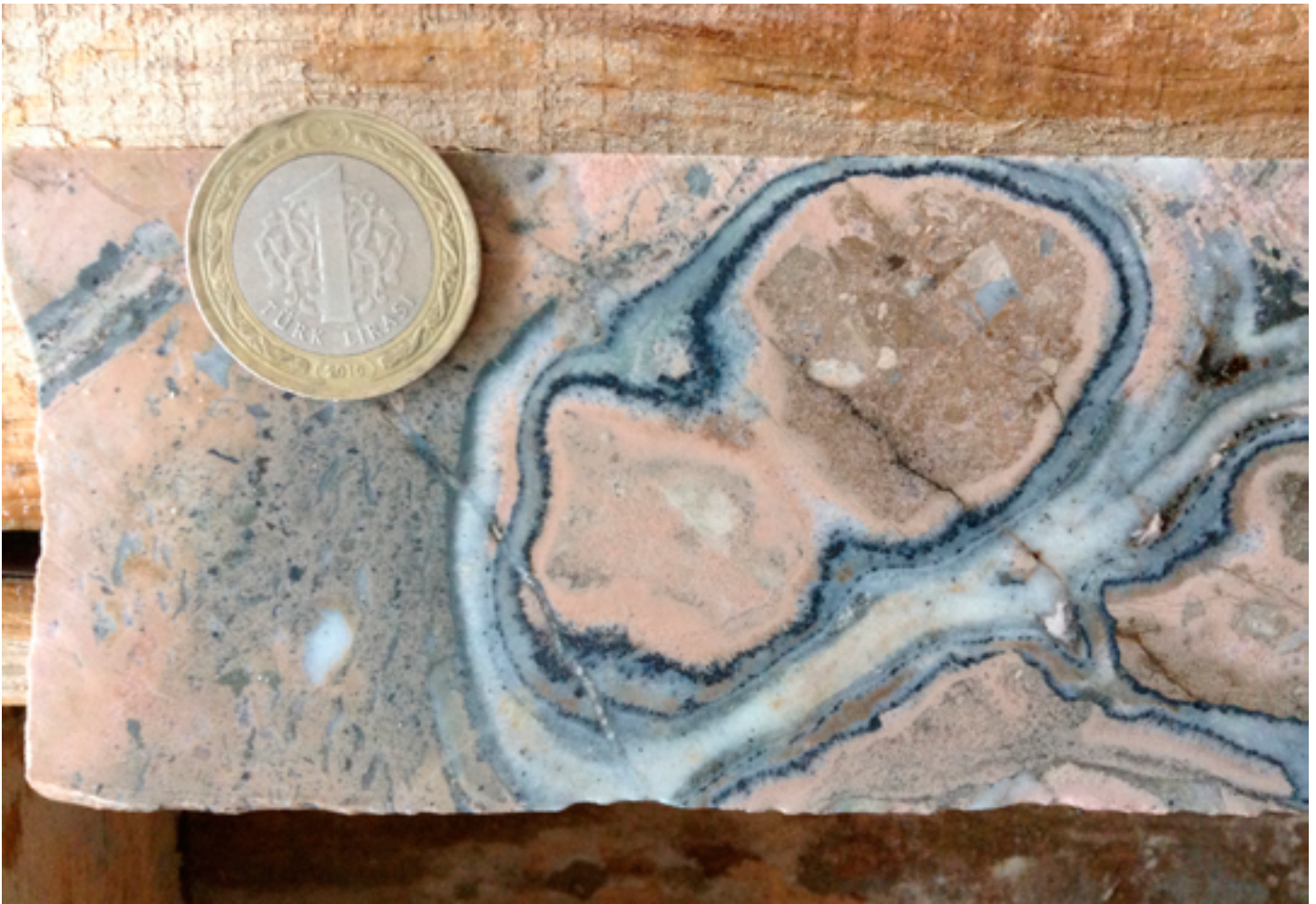
Drill core sample from a gold bearing vein at the Efemçukuru Gold deposit. The sample shows a “cockade texture”, which forms when brecciated clasts in a vein are overgrown by minerals such as quartz (white), rhodochrosite (pink), and sulfosalts (black), which can often contain high-grade gold mineralization.
