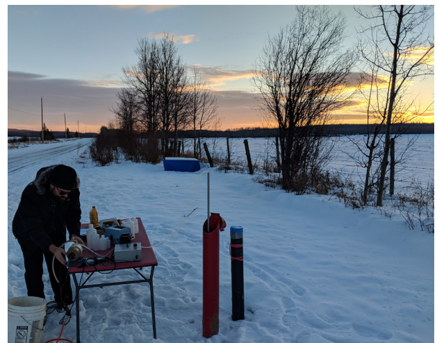
SFU graduate student Andrew Allen samples monitoring wells at the Hudson's Hope Station
